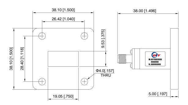
Unit: mm/ inch, General part tolerance is ±2% unless otherwise stated.
