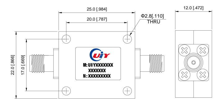
Unit: mm/ inch, General part tolerance is ±0.2mm unless otherwise stated.
