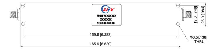
Unit: mm/ inch, General part tolerance is ±2% unless otherwise stated.
