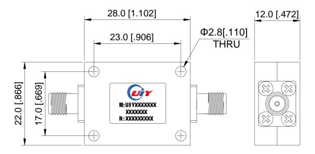
Unit: mm/ inch, General part tolerance is ±0.2mm unless otherwise stated.
