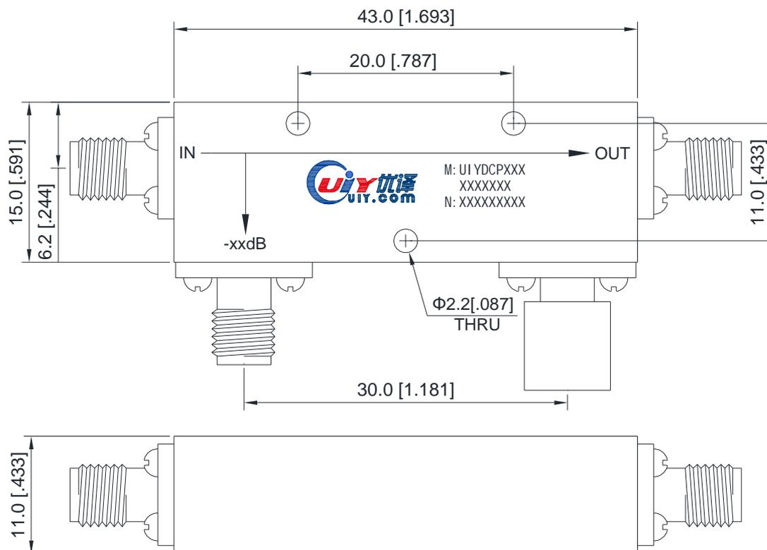
Unit: mm/ inch, General part tolerance is ±2% unless otherwise stated.
