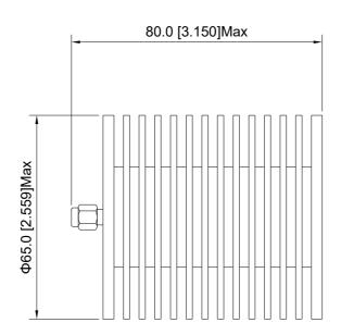
Unit: mm/ inch, General part tolerance is  $\pm 2\%$  unless otherwise stated.
