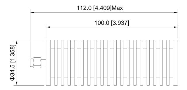
Unit: mm/ inch, General part tolerance is  $\pm 2\%$  unless otherwise stated.
