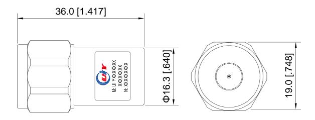
Unit: mm/ inch, General part tolerance is  $\pm 2\%$  unless otherwise stated.
