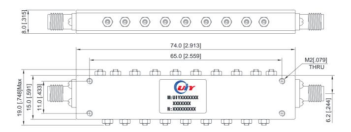
Unit: mm/ inch, General part tolerance is ±2% unless otherwise stated.
