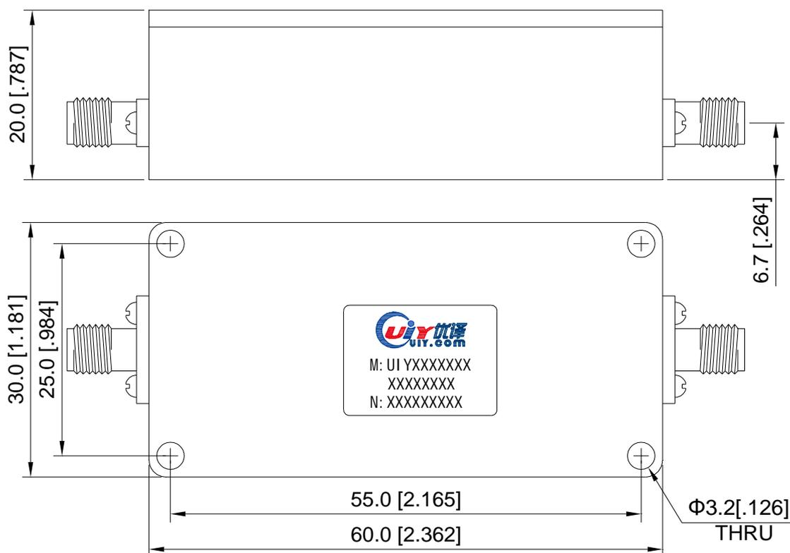
Unit: mm/ inch, General part tolerance is  $\pm 2\%$  unless otherwise stated.
