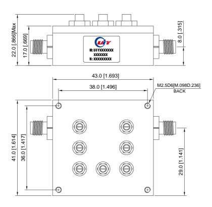
Unit: mm/ inch, General part tolerance is ±2% unless otherwise stated.
