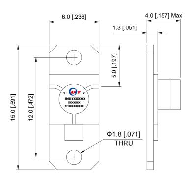
Unit: mm/ inch, General part tolerance is ±0.2mm unless otherwise stated.
