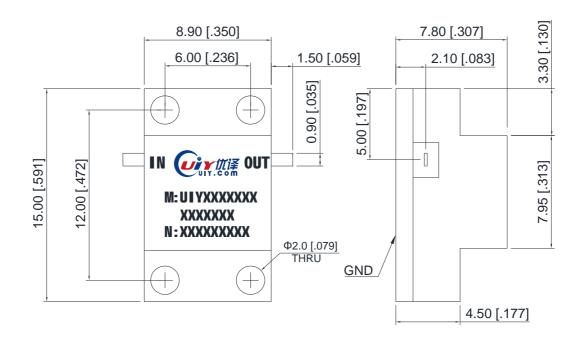
Unit: mm/ inch, General part tolerance is ±2% unless otherwise stated.
