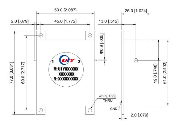
Unit: mm/ inch, General part tolerance is ±0.2mm unless otherwise stated.
