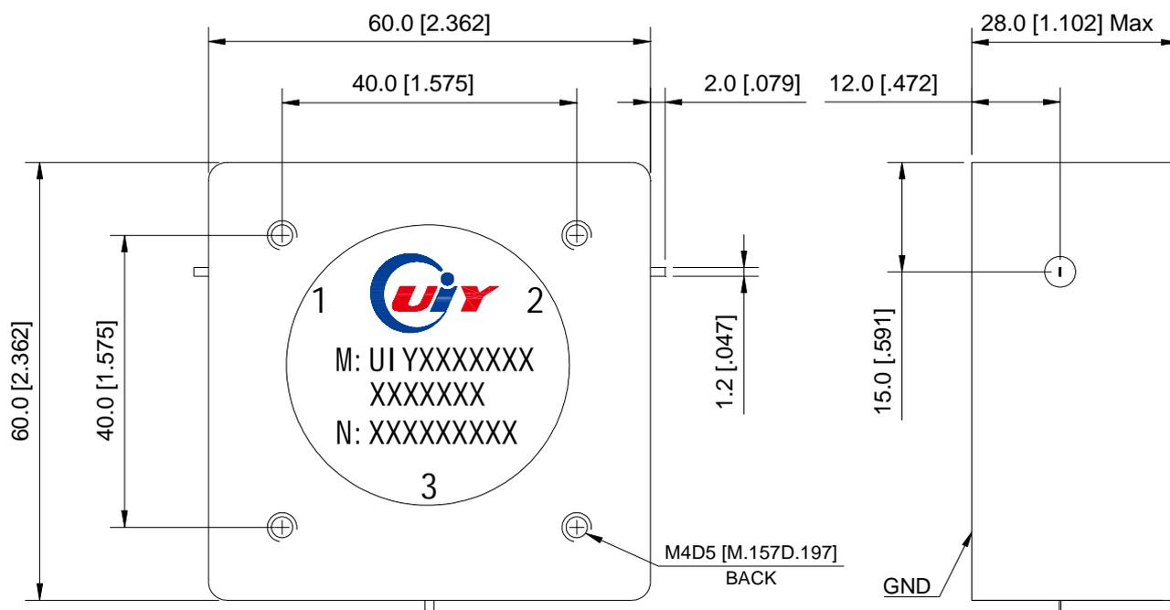
Unit: mm/ inch, General part tolerance is  $\pm 0.2$ mm unless otherwise stated.
