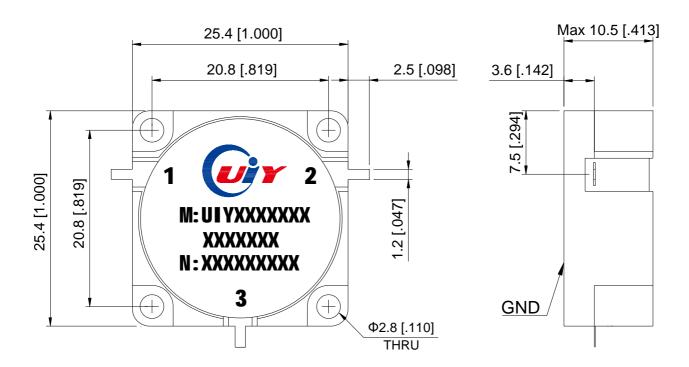
Unit: mm/ inch, General part tolerance is ±0.2mm unless otherwise stated.
