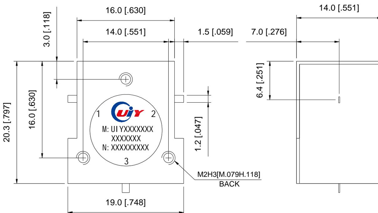
Unit: mm/ inch, General part tolerance is  $\pm 2\%$  unless otherwise stated.
