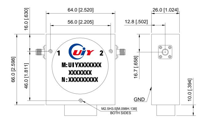
Unit: mm/ inch, General part tolerance is ±0.2mm unless otherwise stated.
