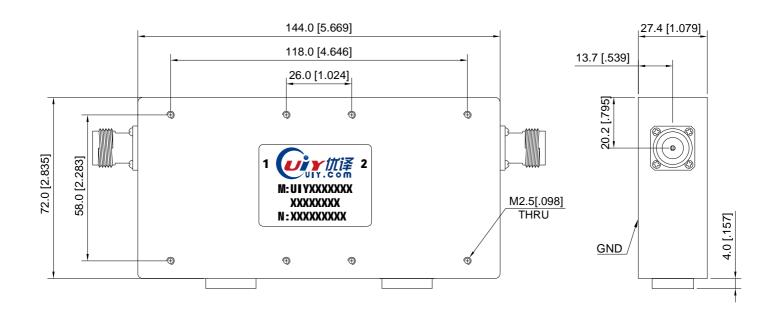
Unit: mm/ inch, General part tolerance is ±2% unless otherwise stated.
