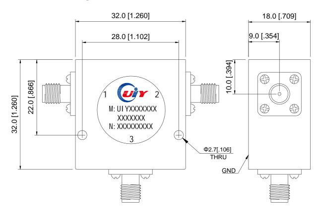
Unit: mm/ inch, General part tolerance is ±0.2mm unless otherwise stated.
