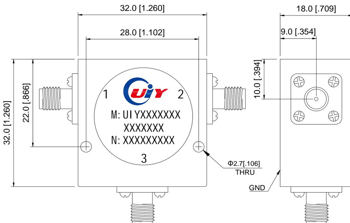
Unit: mm/ inch, General part tolerance is  $\pm 0.2$ mm unless otherwise stated.
