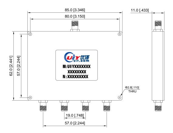
Unit: mm/ inch, General part tolerance is ±2% unless otherwise stated.
