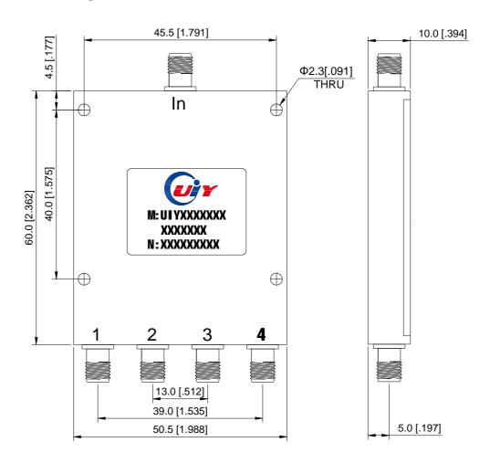
Unit: mm/ inch, General part tolerance is ±2% unless otherwise stated.
