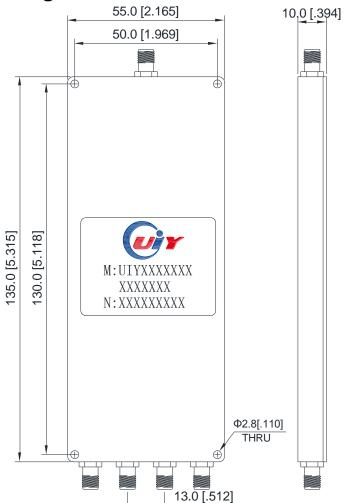
Unit: mm/ inch, General part tolerance is ±2% unless otherwise stated.
