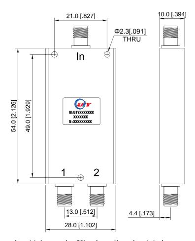
Unit: mm/ inch, General part tolerance is ±2% unless otherwise stated.
