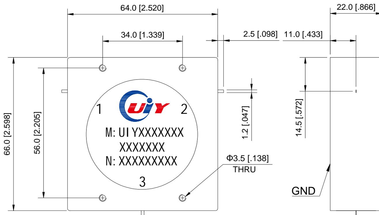
Unit: mm/ inch, General part tolerance is  $\pm 0.2$ mm unless otherwise stated.
