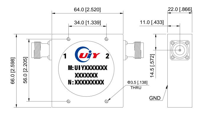
Unit: mm/ inch, General part tolerance is ±0.2mm unless otherwise stated.
