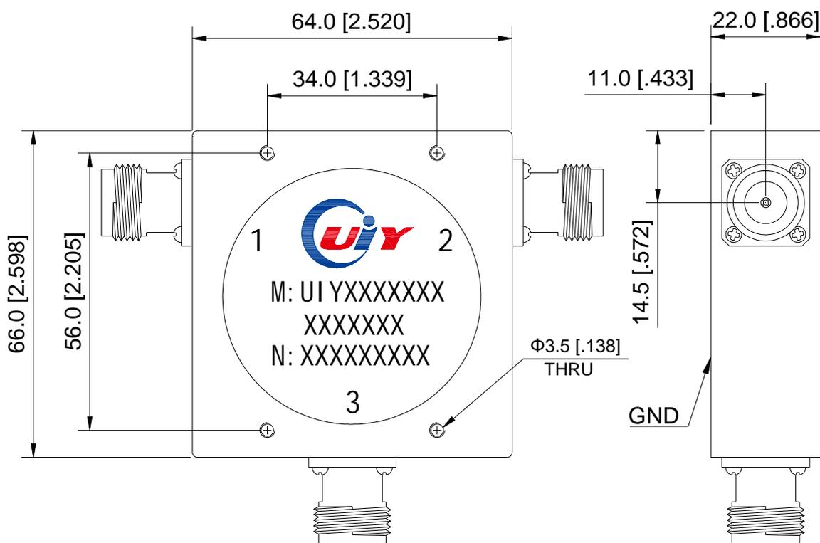
Unit: mm/ inch, General part tolerance is  $\pm 0.2$ mm unless otherwise stated.
